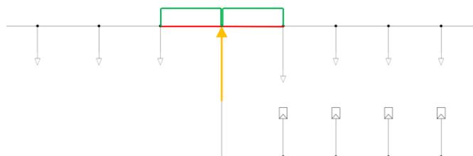
Fig. 9. Parallel cabling with crossing a branching point
